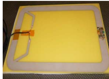
Fig. 2 Printed antenna prototype
