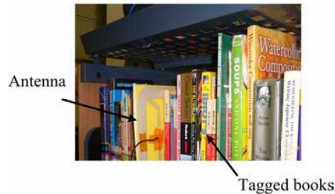
Fig. 5 Implementation of HF Antenna in RFID Smart Shelf
